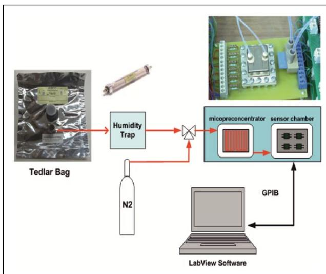
**Figure 1.** A schematic view of the measurement system based on microconcentrator in LTCC technology with gas sensor array based on Figaro sensors.
